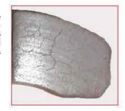
APPEARANCE Pad with surface cracks.
