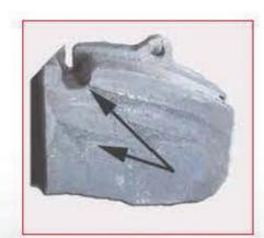
APPEARANCE Excessively worn out discs and pads
