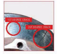
APPEARANCE Disc surface features 1st and 2nd degree crack.
