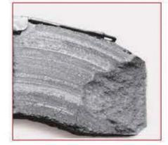
APPEARANCE Detached friction material. Possible excessive load or heavy braking, along with the
