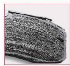
APPEARANCE Contaminated pad friction material.
