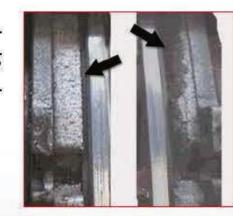
APPEARANCE Damaged edges to the friction material (edge-crumbling).
