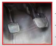
APPEARANCE Clutch pedal remains on the floor
