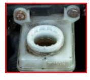
APPEARANCE Abnormal brake pedal behaviour Brown contaminated brake fluid
